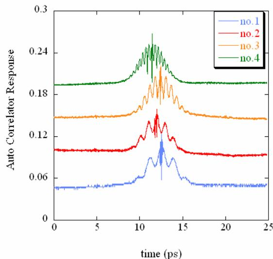
We changed the beating frequency and estimated the laser modulation frequency from the auto-correlator measurement
