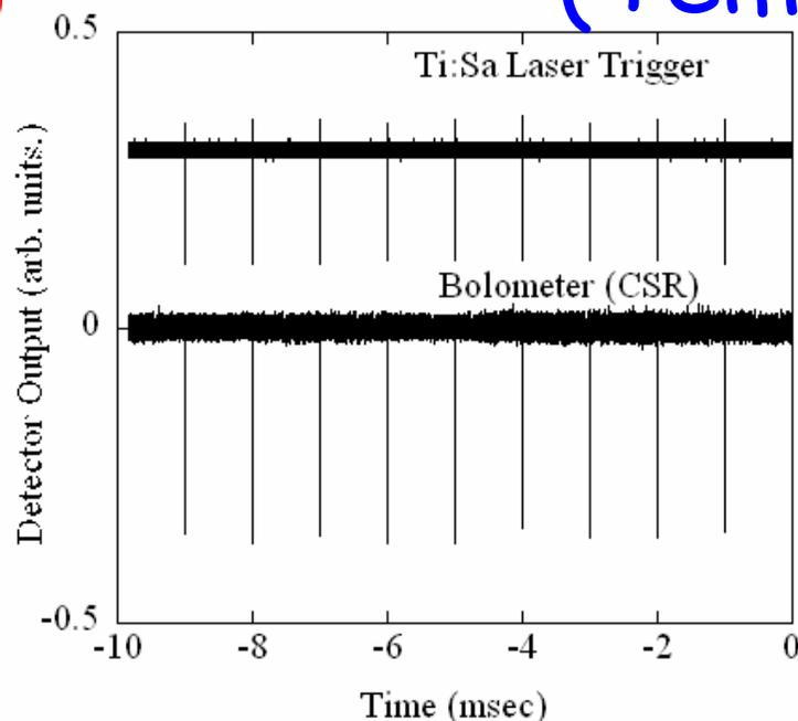
Temporal relation between the laser trigger and THz signal observed at BL6B.
