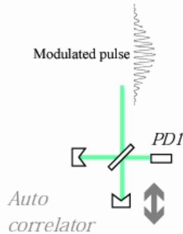
Measurement of the modulated laser pulse with auto correlator
