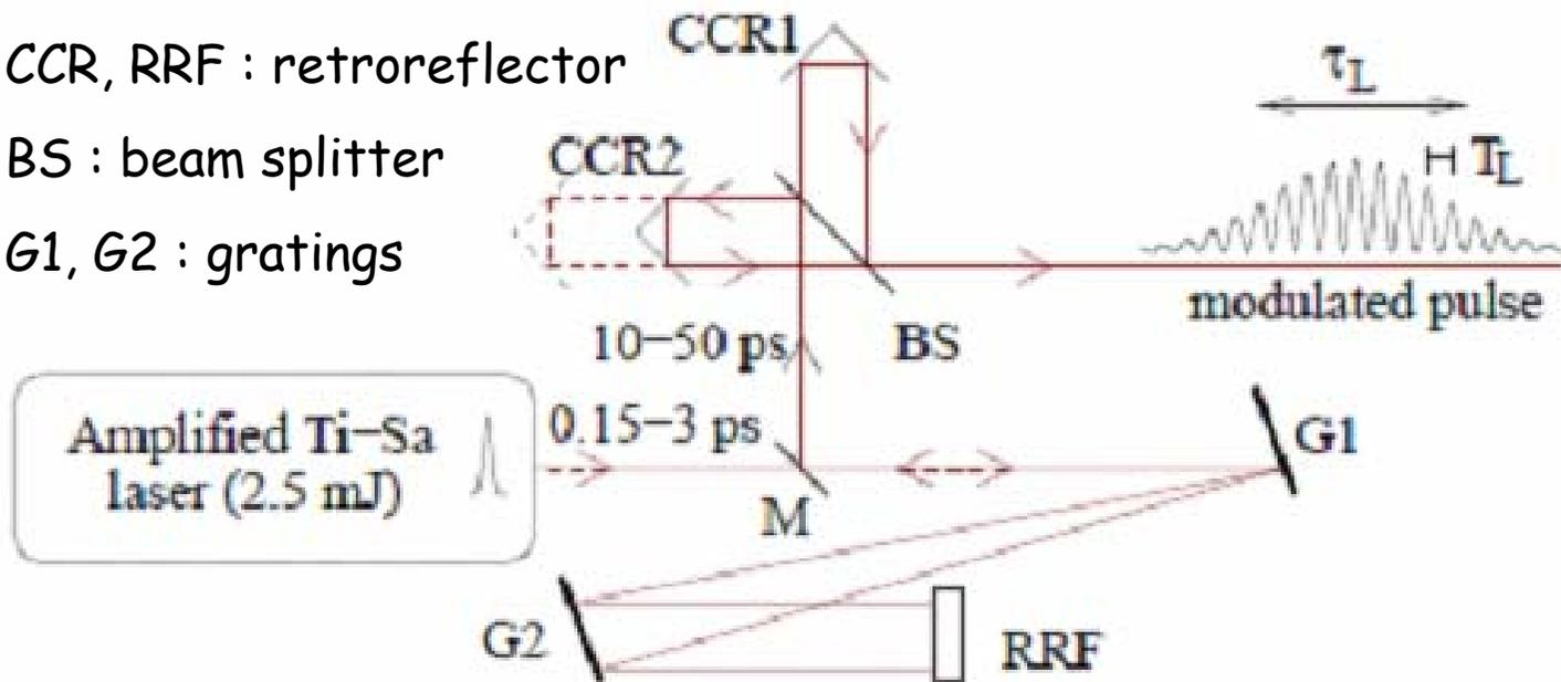
1. Making chirp on the laser pulse with a pair of gratings
