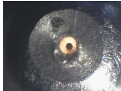
200 μm diameter aperture, 80 μm wire diameter
