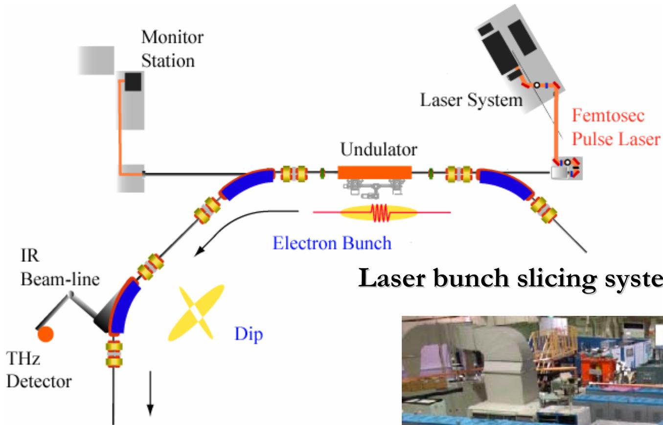
Laser bunch slicing system at UVSOR-II
