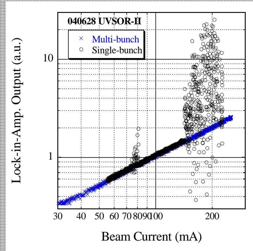
Average intensity of terahertz radiation with a multi-bunch and single-bunch mode
