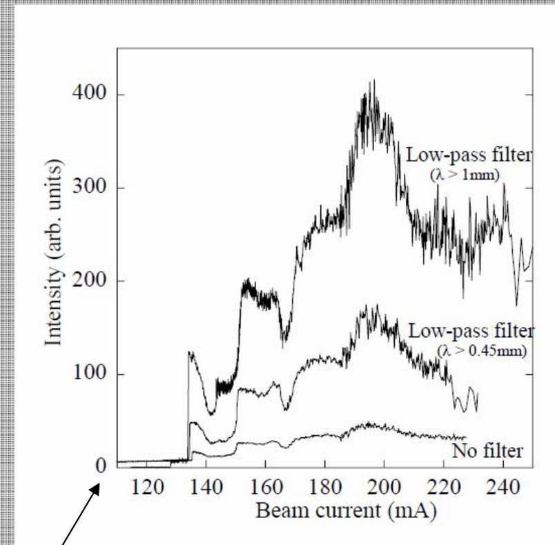
Normalized at the 130 mA, where THz CSR burst does not appear
