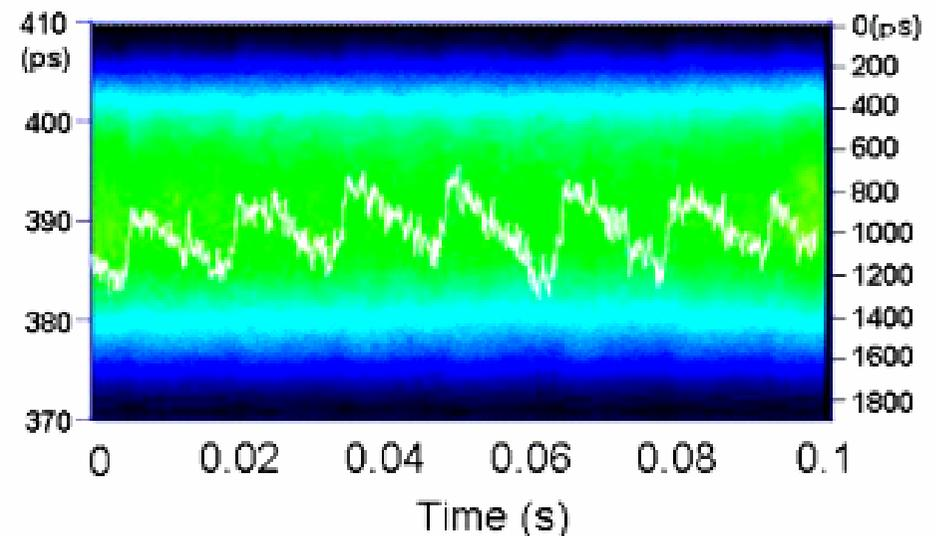
Response of a streak camera synchronized with the signal of the bolometer.
