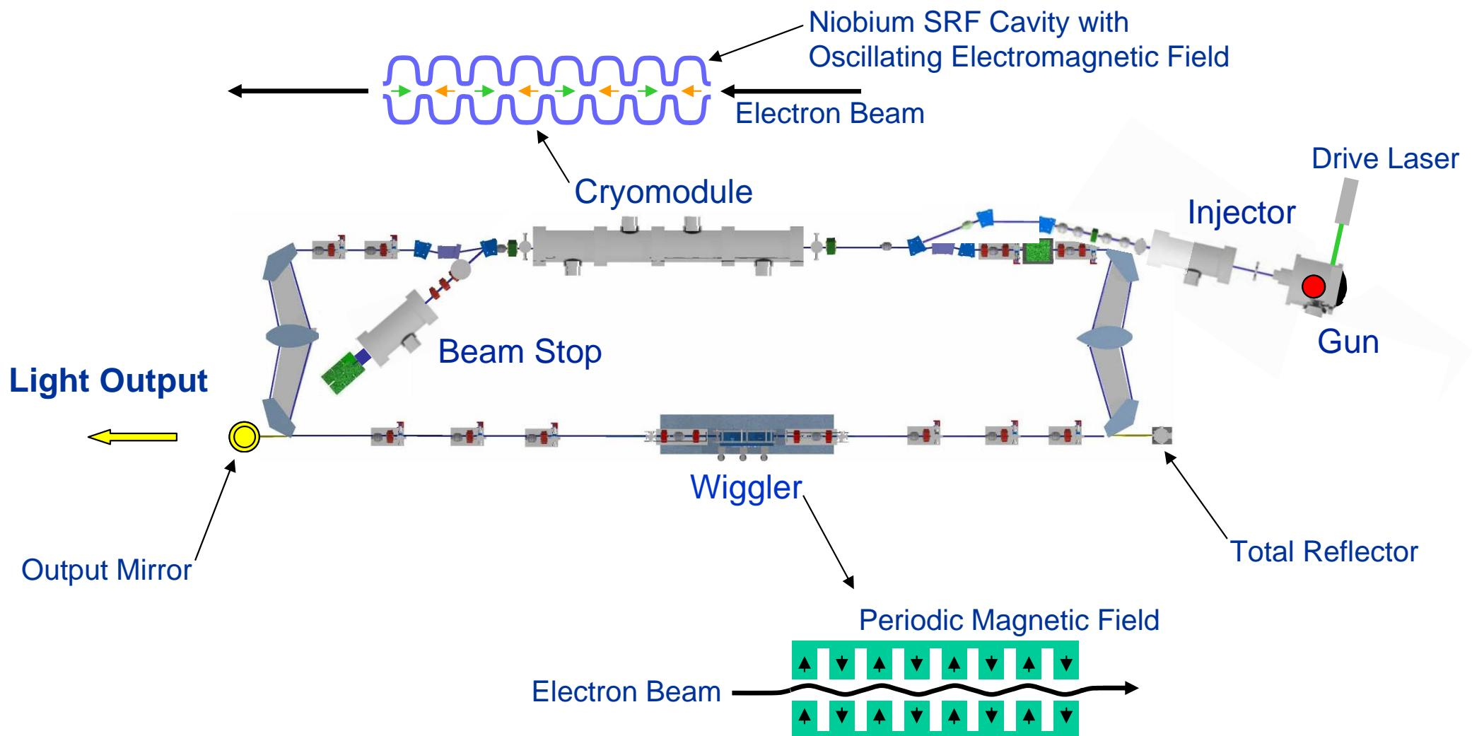
$$\text{Laser Wavelength} \sim \text{Wiggler wavelength}/(2\text{Energy})^2$$
